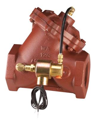
AquaMatic Series Diaphragm Valves are equipped with a 3-way solenoid for direct or remote control. The solenoid can be actuated by a timer, pressure or temperature sensor or liquid-level switch. These valves are ideal for automated process systems.
